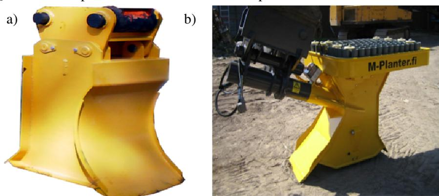
Fig. 2. Devices used for soil preparation: a – MPV-600; b – M-Planter
